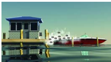
Blockage of boat exhausts by obstruction.
