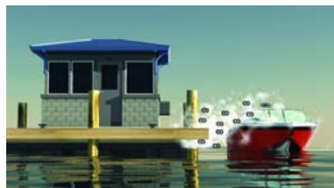
Exhausts traveling along obstruction.
