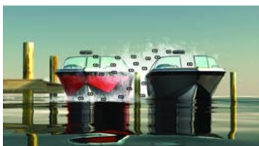
Exhausts from other vessels in confined areas.
