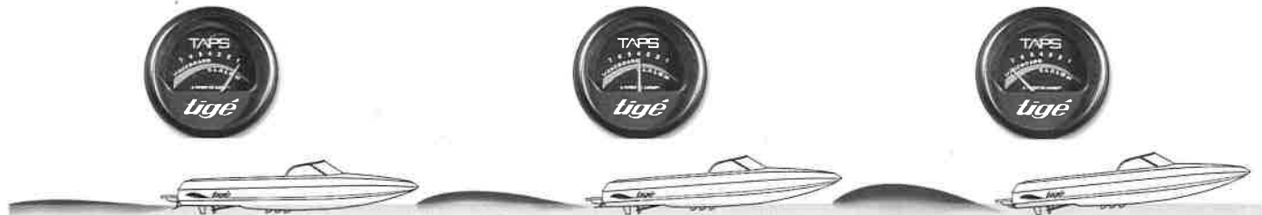
TAPS settings and the effect on hull running attitude and wake characteristics.
