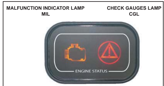
Figure 5-1A Typical Warning Lamp Cluster - CES Engines
